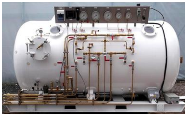
Figure 3: External Decompression Chambers
